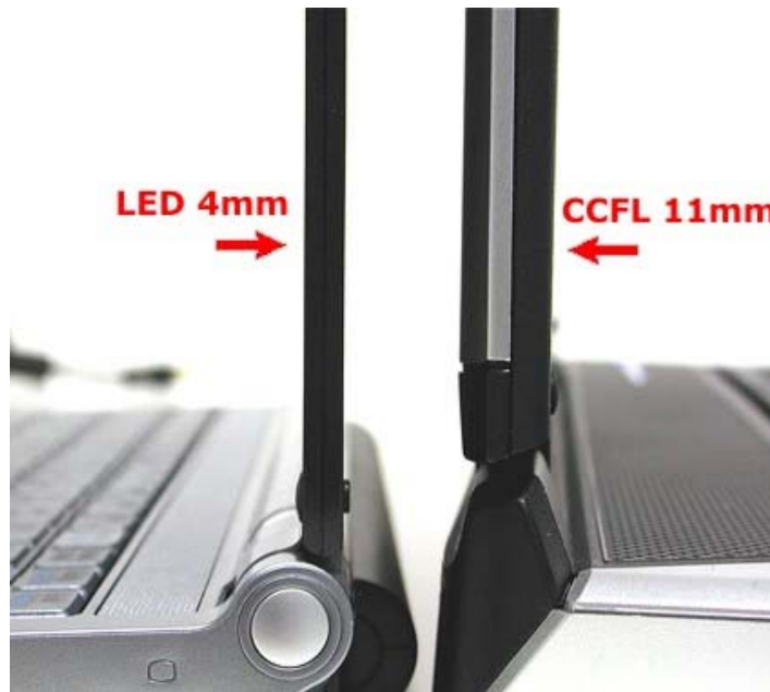
Figure 2 – LCD Panel thickness comparison
