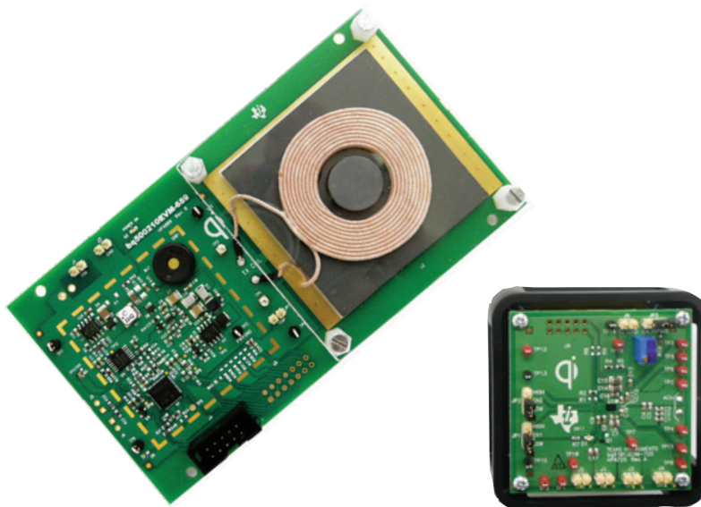
Development kit includes bq500210 and bq51013 evaluation modules.
