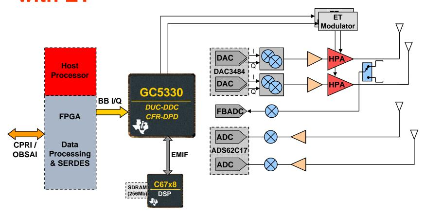
GC5330 This Arch can support 2 x30MHz in HP mode and 2x60MHz in HB mode 24 TX and RX channels (12 channels per ANT)
