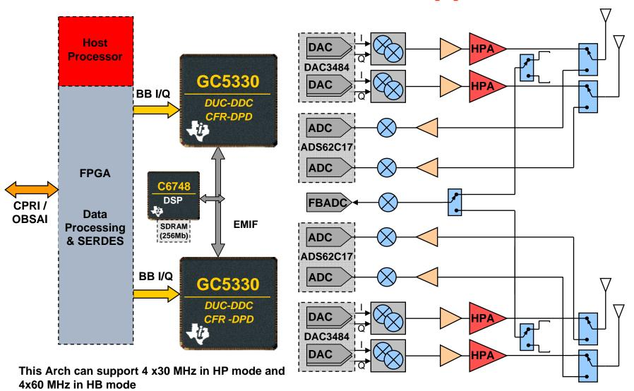
48 TX and RX channels (12 channels per ANT)
