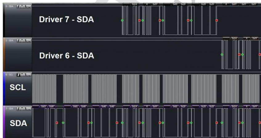
Figure 10. TCA9548A Logic Analyzer Operation
