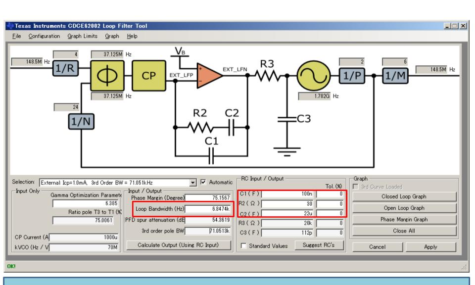
We changed C1,R2,C2 for loop bandwidth. However, we can't set below loop bandwidth of about 7kHz.
