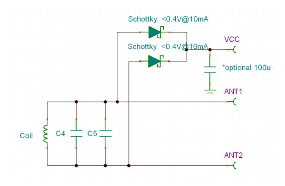
The Coil represents the onboard antenna. C4 and C5 are the antennas resonance capacitors.
