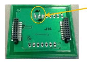
The diodes were soldered on the backside of the board. Make sure to mind the directions in which the diodes are mounted
