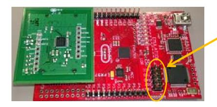
For wireless power operation, all jumpers on the Experimenters Board have to be disconnected!
