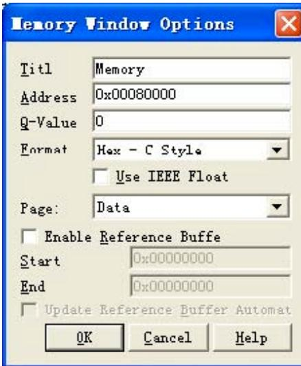
After pressing OK, you will see the following screen, if the values increases from 0X0000 to 0X3FFF, it means the external RAM is fine, otherwise please check on the external RAM.
