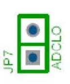
When ADCLO Jumper is in jumpering, it is internal AGND input; when not in jumpering, it is JP1 or JP2 bus ADCLO pin, input external AD sampling signal's ADC earth level signal.
