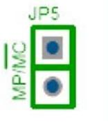
MP/MC Jumper, when debugging, not in jumpering, JP5 is in MP mode. When downloading Flash, JP5 is in jumpering, it's in MC mode.
