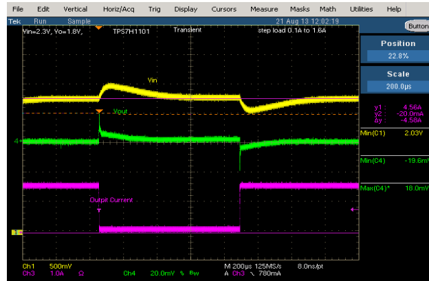
Figure 25. Load Transient Response: Step Load 0.1 A to 1.6 A, V_{IN} = 2.3 V, V_{OUT} = 1.8 V (TPS7H1101-SP)
