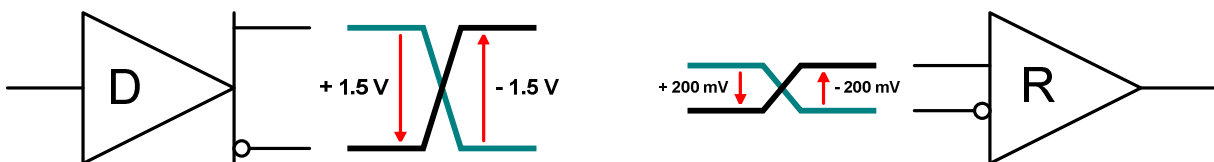
Figure 2. RS-485 specified minimum bus signal levels
