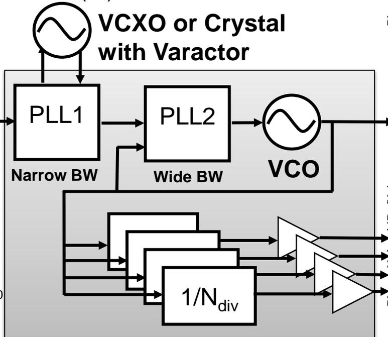
CLKout is a cleaned, low jitter replica of the reference clock.
