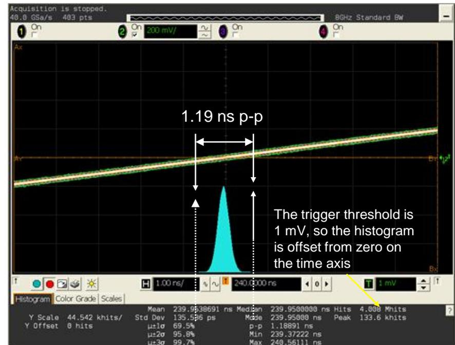
Even 40 GS oscilloscope is not recommended for measuring 316 fs of random jitter!
